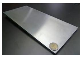
Figure 3: A FAST/SPS-sintered sputter target made of a technical ceramic with a 2-Euro coin lying on it for size comparison.
