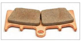
Figure 6: Motorcycle brake lining. Copper-plated carrier (bottom) and two sintered friction linings. The two materials are bonded during sintering without the use of auxiliary materials, and the sintering of the friction lining does not require any subsequent calibration.
