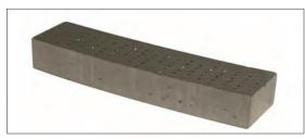
Figure 1: Typical diamond tool segment consisting of a metal matrix in which diamonds are embedded in defined positions and several layers by means of a technique developed by Dr. Fritsch ("DiaSet"). These segments are, for example welded onto cut-off wheels or drill bits, used for cutting asphalt, granite, marble or concrete.
